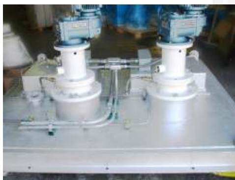
Figure 8 Process gas dispersers shown on two rotor tilting degassing system. LARS™ HF Series.
