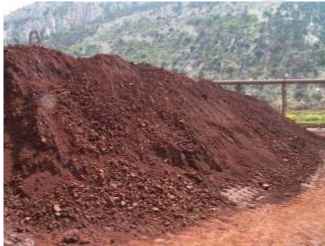
Fig. 2. Red mud filter cake obtained by plate and frame filter press
