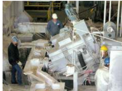
Figure 4 Almex LARS™ HF degassing system in end of cast tilting mode.
